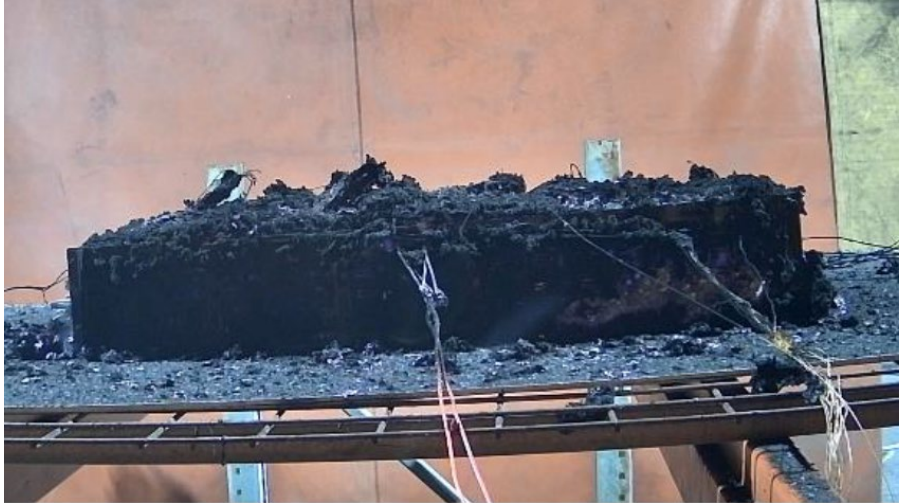
Figure 6: Samsung SDI Module MS1304E101A UL9540A Module Level Test Result.
